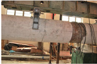
图2 试件的破坏形态及裂缝分布 Fig.2 Failure mode and fracture distribution of specimens
