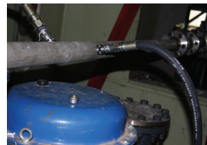
图 7 示踪粒子注入主气流 Fig.7 Injection of tracer particle
