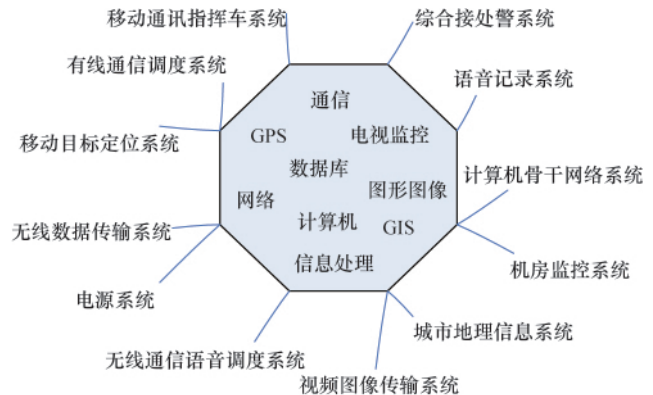
图 1 城市应急联动系统技术及功能组成 Fig. 1 Technology and functional components of city coalition emergency response system
