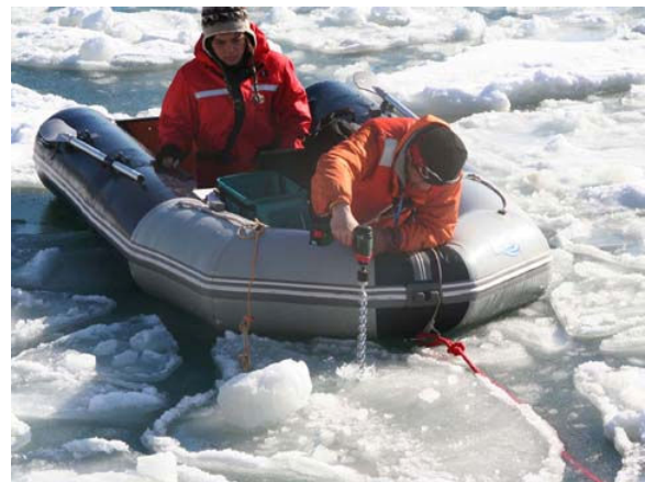
(a) Opening a hole on the ice with a drill.
