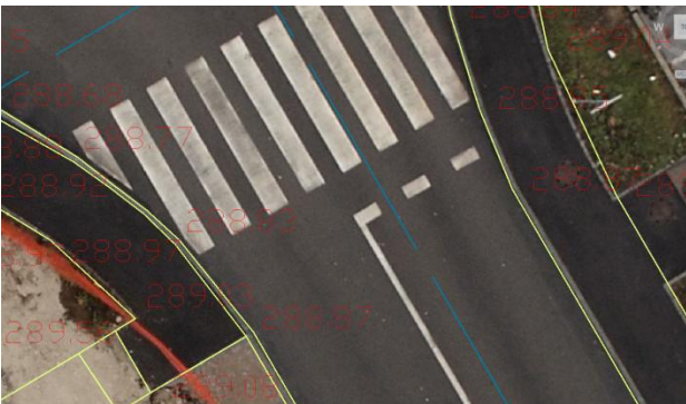
Figure 5. A subset of comparison of photogrammetric (ortho-photo) and control measurements
