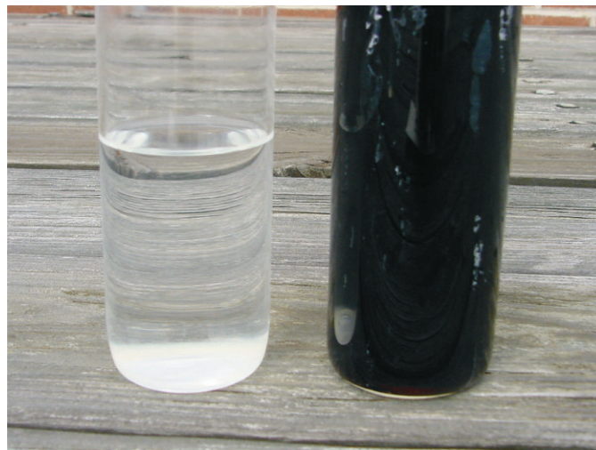
Fig. 1. The leachate after 459 d of exposure to solar radiation on a roof (left) and the dark control leachate treated similarly except wrapped in aluminum foil (right). The absorption spectra of CDOM are shown in Fig. 2.
