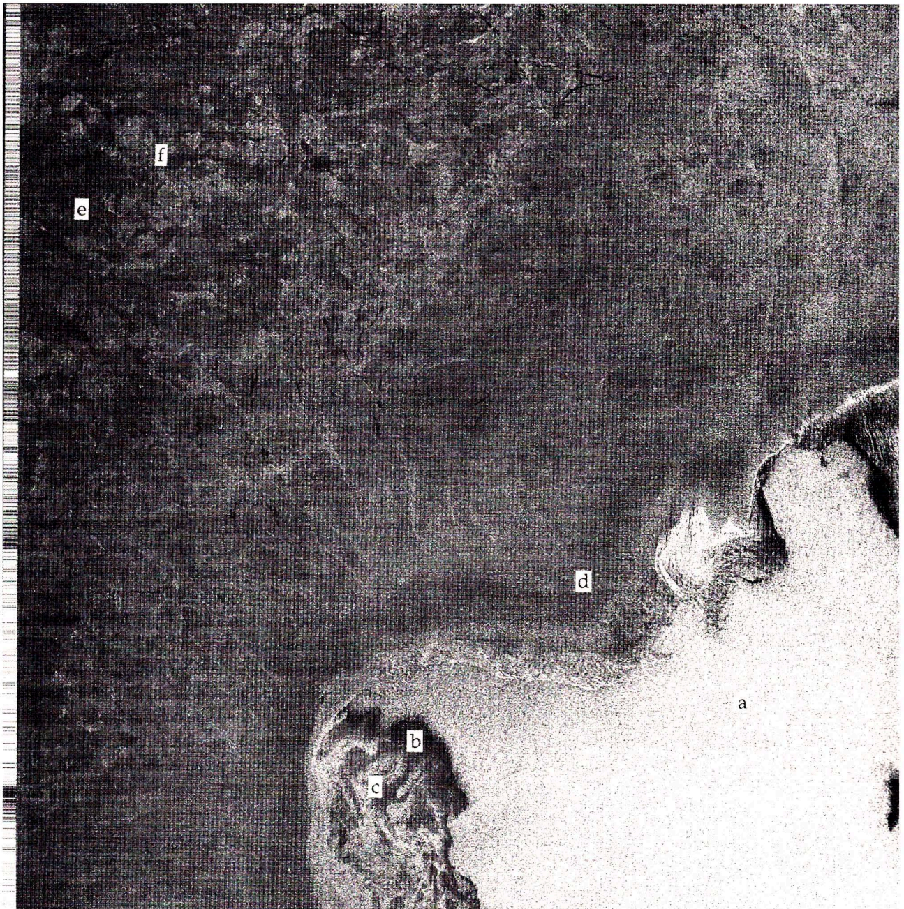
Fig. 3 - ESR-1 SAR image covering 100 x 100 km of the experiment area obtained on March 5. The image shows open water (a), grease ice (b), pancake ice (c), uniform field of 2 - 3 m thick broken-up firstyear ice (d), consolidated firstyear ice in the interior of the ice pack (e), and multiyear floes (f)
