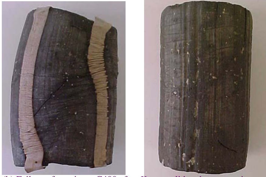
(b) Failure of specimen C400 after K_o -consolidated compression testing and (c) failure of specimen E400 after K_o -consolidated extension testing
