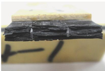
(b) Z-pin reinforced laminate (insertion pattern C)
