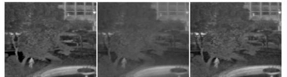
(a)对比度金字塔融合 (b)加权平均融合 (c)拉普拉斯融合 (a)Contrast Pyramid fusion (b)Weighted average fusion (c)Laplace fusion
