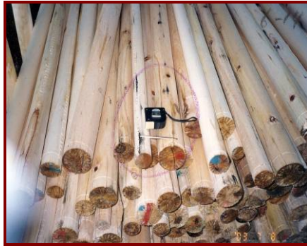
Photos 36 : use of old fashioned rotary resulting in large cores
