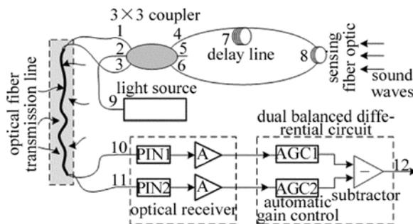
Fig. 1 The anti-disturbance type all fiber-optic interferometer system
