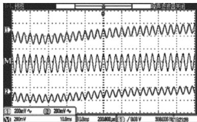
Fig. 5 Experimental result of interferometric optical fiber acoustic sensor
