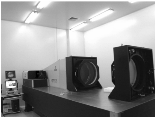
图2 \phi 600 mm大口径双端口数字平面干涉仪 Fig.2 \phi 600 mm digital laser interferometer
