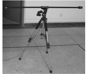
(b) 一维基线尺靶标 (b) 1D target with known precise length
