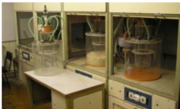
Fig. 4. View of the laboratory device. The big plastic contains has inside a material of the litter, wood-shavings (see the container in the middle). Another container, on the table before a fume chamber, shows the measuring sensor. It is placed on the top of the container. The workplace involves measure four samples at this time
