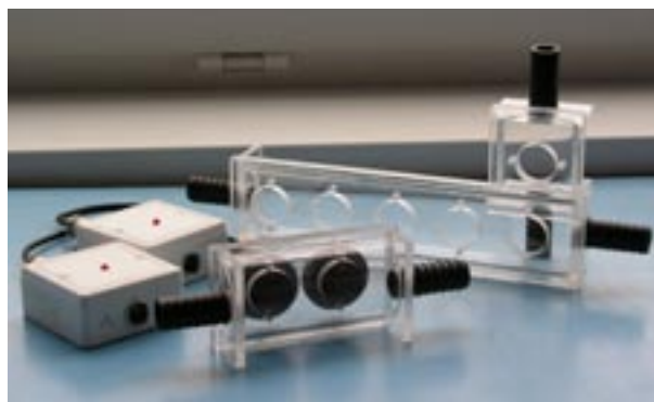
Fig. 5. Housing of two sensors in one case is at front. Two small white boxes on left part in the figure consist auxiliary electronic circuits of the sensors. The case is for housing one sensor and next too empty case for five sensors you can see at the back the figure. The case with five sensors was used for their calibration. Standard measurement of ammonia concentration is done with two sensors in one case
