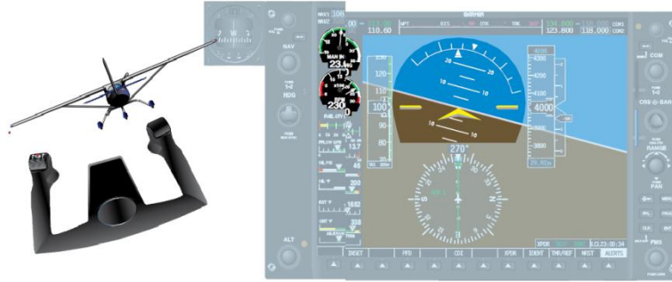
Fig. 1) The screen depicting some of aircraft's control instruments (pitch=0°; bank=15°) [1]
