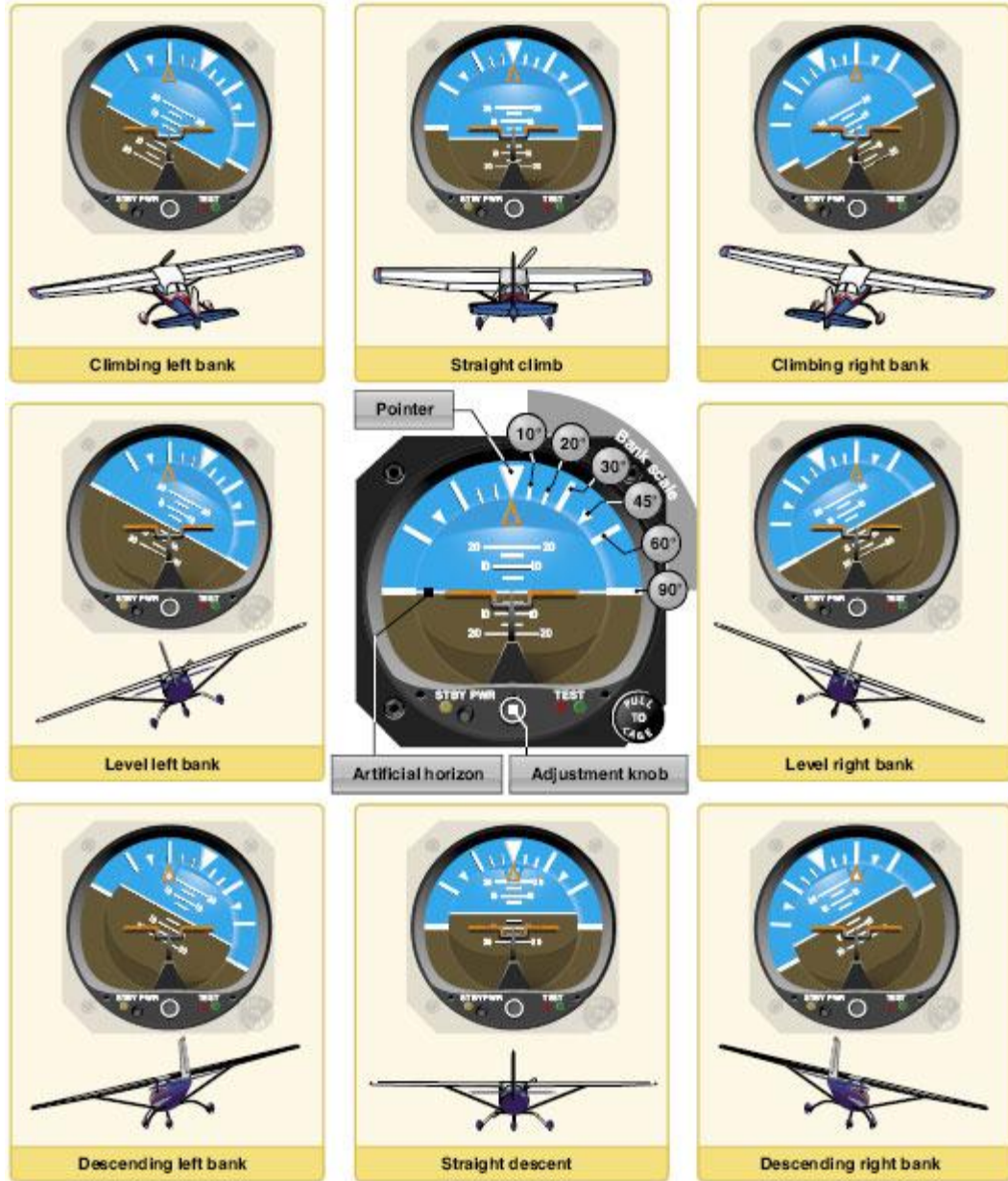
Fig. 11) Interpretation of Attitude Indicator readings [14]
