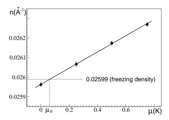
FIG. 12: (Color online). Liquid density as a function of chemical potential at low temperature T=0.25 K. The slope of the solid line is deduced from the simulated values of compressibility averaged over four points shown in the plot. The critical value of the chemical potential deduced from this plot is estimated as  $\mu_{\circ}=0.06\pm0.04$ .
