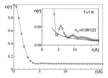
FIG. 8: One-particle density matrix n(r) for N=1024 particles at T=1~K and SVP pressure. The solid line is the theoretical prediction based on the long-wave phase fluctuations, Eq. (6.1).
