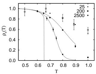
FIG. 5: Superfluid fraction  $\rho_s(T)$  computed for 2D <sup>4</sup>He on systems with different numbers N of <sup>4</sup>He atoms. The system density is n=0.0432 Å<sup>-2</sup>. Dashed lines represent fits to the numerical data (in the critical region) obtained using the procedure illustrated in Ref.<sup>25</sup>. The leftmost dashed line is the extrapolation to the infinite system. Open squares show results obtained in Ref.<sup>25</sup> for the same system, with N=25.
