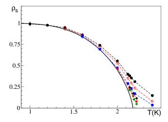
FIG. 9: (Color online). Superfluid fraction  $\rho_s(T)$  as a function of temperature at SVP, computed for different system sizes, namely N=64 (filled circles), N=128 (open circles), N=256 (filled squares), N=512 (diamonds), N=1024 (triangles down), and N=2048 (triangles left). The solid line is the experimental curve.
