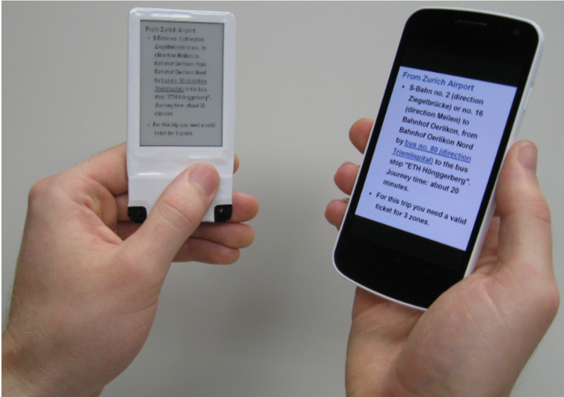
Figure 6.1. One application of the display tag is a companion display for a mobile phone. The pixelated NFC display tag on the left mirrors the travel directions shown on the screen of the phone on the right. The power and data required to update the display are provided by an NFC connection between the tag and phone.
