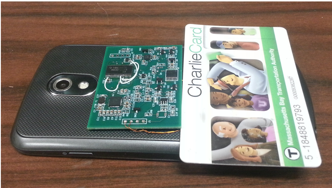
Figure 5.10. Our EnGarde prototype meets the form factor needs required for semi-permanent attachment to a mobile phone. Here, we show it on the back of a Galaxy Nexus
