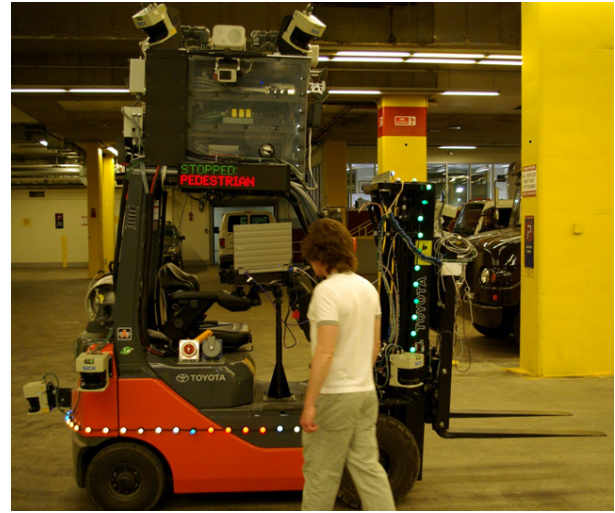
Fig. 9. The forklift detects an approaching pedestrian and pauses. Colored lights skirting the vehicle indicate the proximity of close objects (red to green lights map range from close to far). The LED signs display the reason for pausing.
