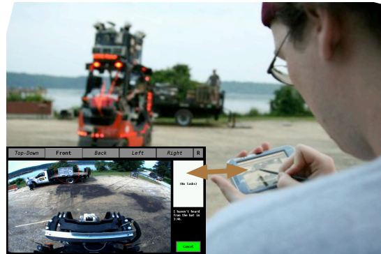
Fig. 1. The supervisor commands the forklift to lift a pallet from a truck, by circling the pallet on the robot’s-eye-view displayed on the tablet interface (inset). The tablet also interprets simple spoken commands to summon the forklift to various task areas within the warehouse.
