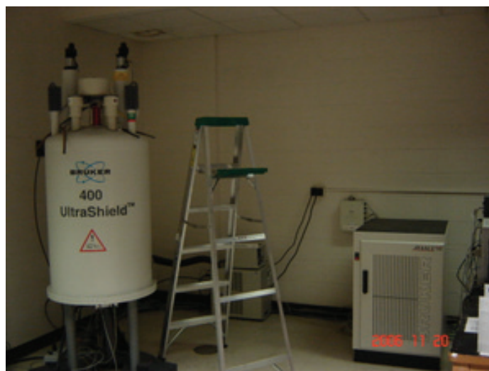
Figure 5.3. UMass Amherst’s NMR facility Bruker Avance400 Spectrometer with 400 MHz RF source, 9.4 T liquid helium cooled superconducting magnet, variable temperature control unit, and XYZ-gradient probe.
