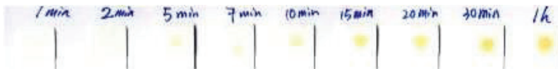
Figure 4.4 Digital images of a sequence of test strips exposed under increasing time for a solution containing 100 \mu\text{g L}^{-1} of arsenic
