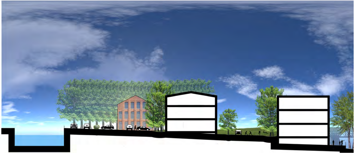
This section is cut between the Merrimack River and the South Canal looking West. It cuts through the South Canal, South Canal Street, a parking lot, a residential building, a woonerf, another residential building, the Merrimack River Trail, and the Merrimack River.
