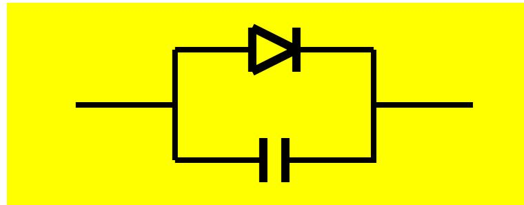
PN junction capacitance { Depletion capacitance  $C_T$
