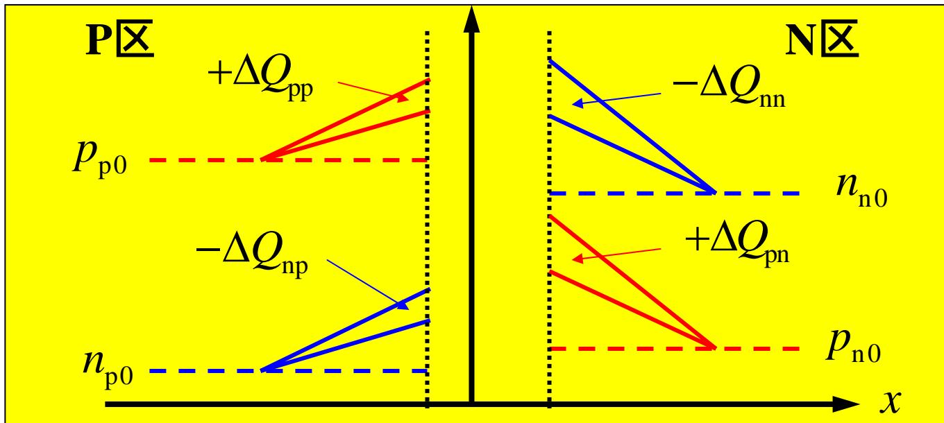
$$V_1 = \Delta V \rightarrow \begin{cases} \text{N region : } +\Delta Q_{pn} \text{ (simultaneously } -\Delta Q_{nn} \text{)} \\ \text{P region : } -\Delta Q_{np} \text{ (simultaneously } +\Delta Q_{pp} \text{)} \end{cases}$$
