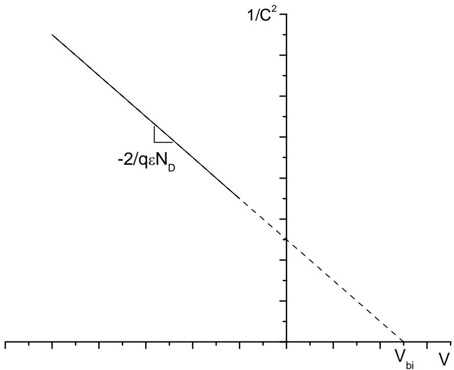
A capacitance versus voltage measurement can be used to obtain the built-in voltage and the doping density of a one-sided p-n diode. The capacitance-voltage characteristic and the corresponding  $1/C^2$  curve are shown in the left figure.
