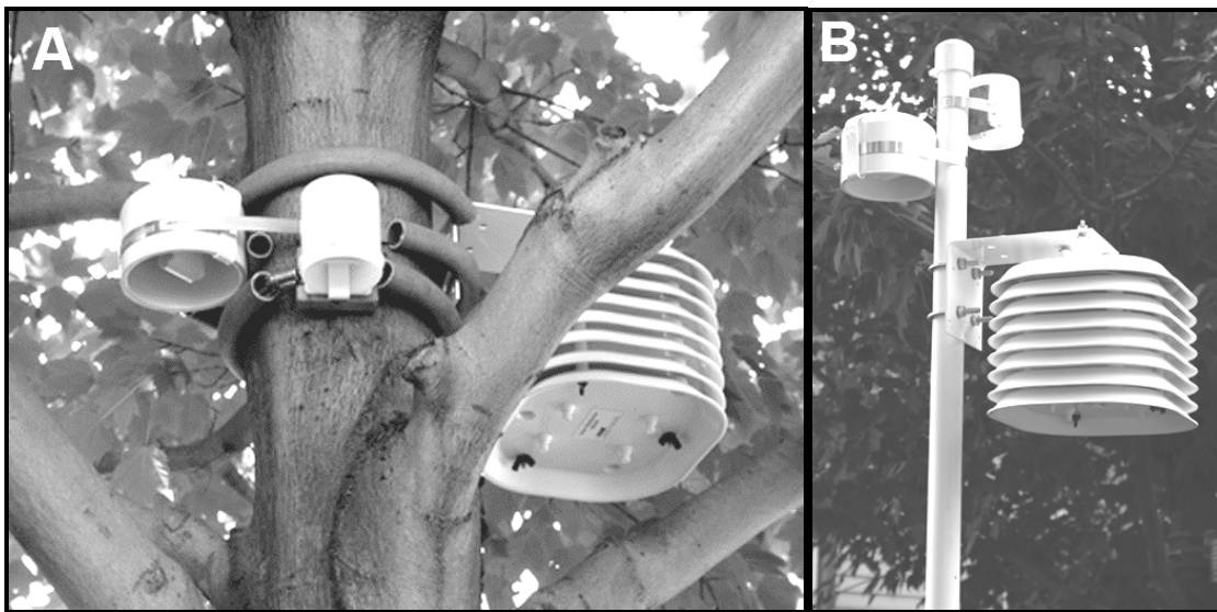
Figure 4.2. Setup of O 3 and NO 2 passive samplers inside rain shelters and temperature/RH logger inside solar radiation shield (left to right, respectively within each image) for inner (A) and outer (B) canopy locations.
