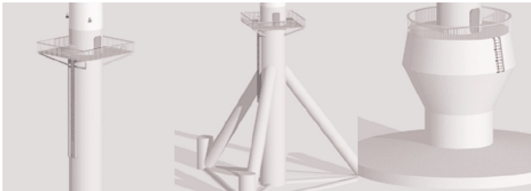
Figure 4 – Offshore wind turbine structures for shallow water. From L-R: monopile, tripod, and gravity foundations [60]
