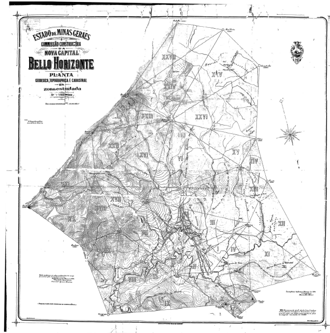
Figure 3.1 “Bello Horizonte – Geodesic, Topographic and Cadastral Map of Area Studied.” This map displays the triangulations upon which Reis would base his street grid. Notably, his design ignores the topographic elements contained here. Hermillo Alves, engineer and B. Zickler, designer. 1895. Photo courtesy of the Arquivo Público Mineiro.
