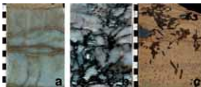
Figure 2. Core sampling of clearly identified evaporite facies within the sediments of the Michigan Basin. Scale bars are in centimetres. a) Regularly bedded anhydrite after gypsum (relics of «grasslike» crystal beds, now anhydrite). Usually formed just below the pycnocline. Allecco Prins #1-16 core at 2432 feet (741 m) Allegan Co. (MI); Devonian; b) Clear relic outlines of twinned gypsum crystals, now massive anhydrite. Dark colour is caused by organic-rich clay that lay between original gypsum crystals. Summit-Anderson #131 at ~4300 ft (1310 m), Isabella Co. (MI); M. Devonian (Richfield Member); c) Typical anhydrite replacement of carbonates. Dark grey colour represents anhydrite replacement of carbonate. White nodule represents both infilling of a void plus replacement by anhydrite. Allecco Prins #1-16 core at 2463 feet (750.7 m), Allegan Co. (MI); Devonian.
