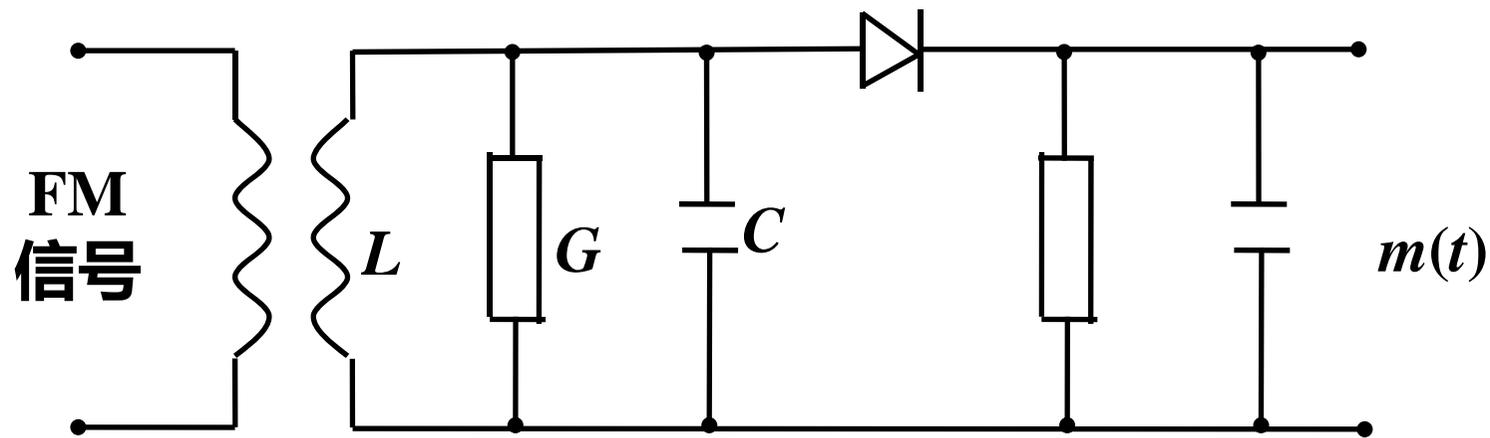
$$|H(\omega)| = \left| \frac{V_0(\omega)}{I(\omega)} \right| = \frac{1}{G} \left[ 1 + \left( \omega C - \frac{1}{\omega L} \right)^2 / G^2 \right]^{-\frac{1}{2}}$$
