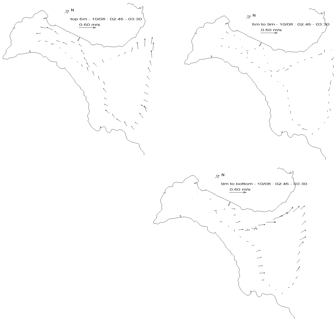
Fig. 7 Observed currents in surface, middle and bottom layers during flood tide
