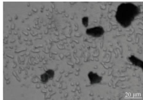
(h) High magnification of  $Ti_{45.5}Ni_{45.5}Al_9$  after erosion
