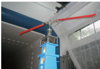
图4 模型旋翼在旋翼台上的试验布置 Fig.4 Experiment layout of model rotor on rotor test rig
