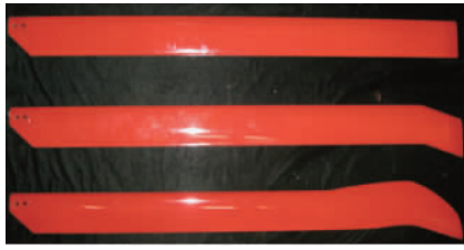
图2 3种模型旋翼桨叶对比 Fig.2 Comparison of three model rotor blades
