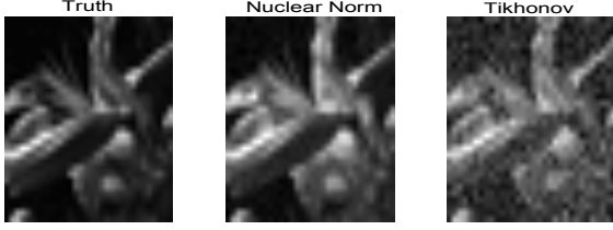
Fig. 5. This figure shows an example of the true image, low-rank reconstruction, and least square reconstruction, from the hyperspectral flower at band 12.
