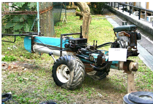
Figure 2. VAKIMPAK, a mechanical striking seismic source used in the field for generating P- and S-waves. The striking energy is much stronger than the sledgehammer, about 2500 Nm for P-wave and 2000 Nm for SH-wave.
