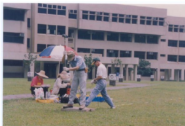
Figure 3. Shear wave generating by using a sledgehammer striking against the end of a block of a wooden plank.
