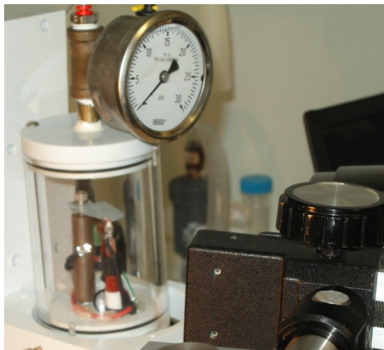
Figure 18. Pressure chamber used to test the effect of pressure on corona discharge.
