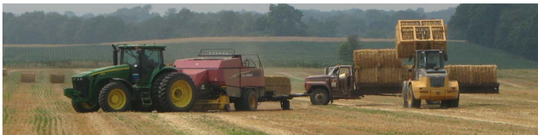
Figure 1. The large square baler, bale handler, and bale truck used in straw harvesting.
