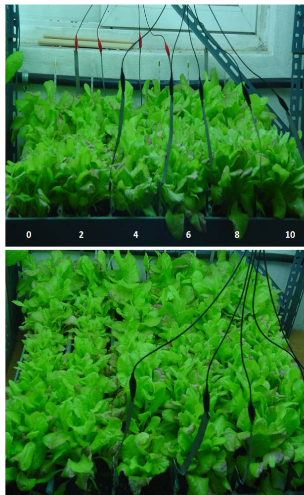
Figure 4. Side view (upper) and wide view (lower) of lettuces cultivated in conventional culture soil (0 V) and 2 - 10 V of the electrically pulsed culture soil for 42 days.
