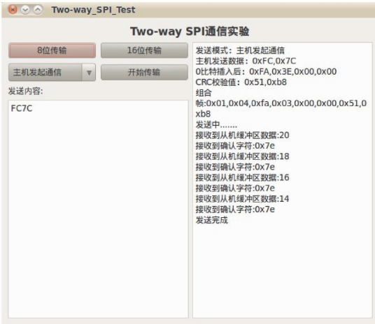
图 10 主机发起 two-way SPI 通信的测试情况 Fig. 10 Test case for two-way SPI communication launched by host
