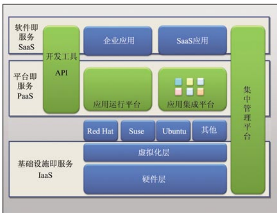
图 2 云计算实施架构 Fig. 2 Cloud-computing implementation architecture
