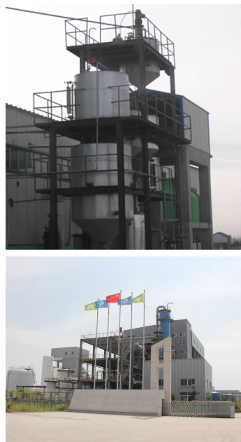
Fig. 2 Industrial lines of carbon dioxide based polymers: upper, the pilot line of Mengxi High-tech Group (2004); lower, the 30000 ton/year production line in Zhejiang Bangfeng Plastics Company (2012).
