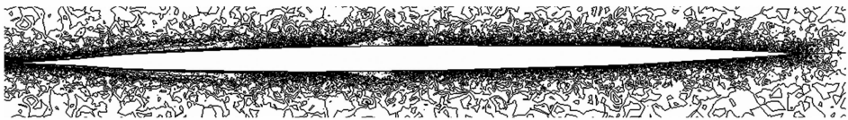
图5 赛艇周围的等压线图 ( B=4.54 ) Fig. 5 The pressure contour around rowing ( B=4.54 )
