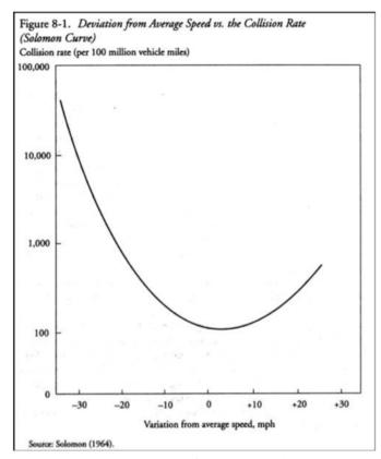
Figure 2: Solomon's curve deviation from average speed and collision rate.
