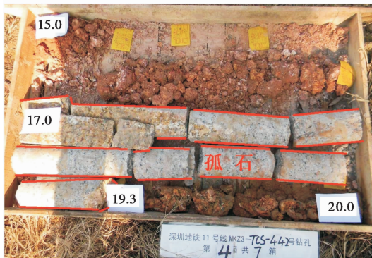
图5 442 号验证孔揭示的花岗岩孤石岩心 Fig. 5 Appearance of boulder in a core recovered from borehole 442
