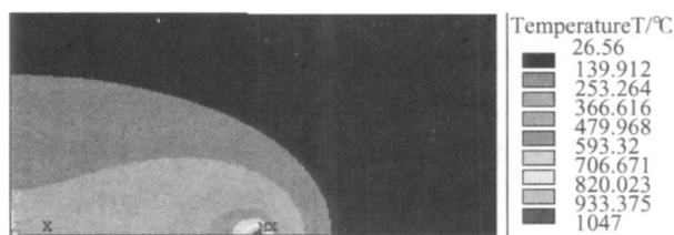
图 2 焊接过程持续 55 秒时温度分布云图 Fig. 2 Nephogram of temperature distribution at 55th second of welding process
