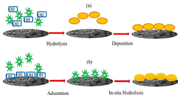
**Scheme 1** Schematic of the two formation modes of the photocatalyst.
