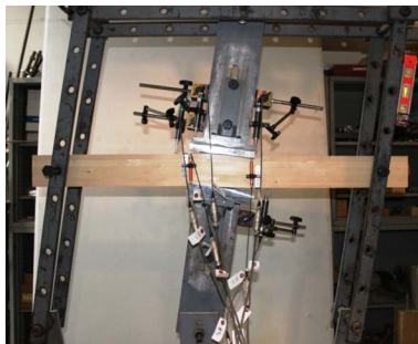
Figure 15. Continuous beam rotated by 0.005 rad.
