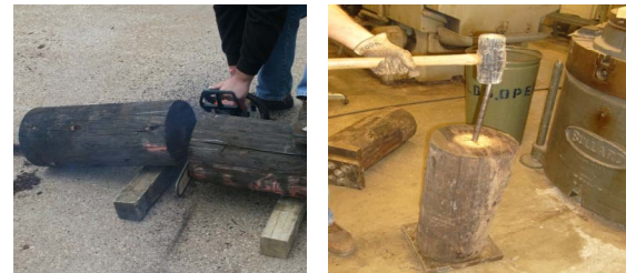
(a) Pile cutting
