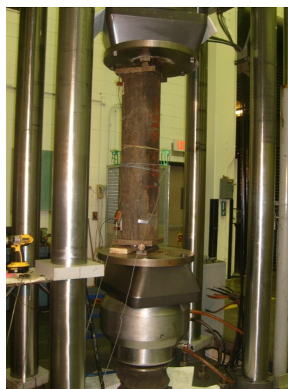
Figure 11. Installed specimen in the MTS testing machine.
