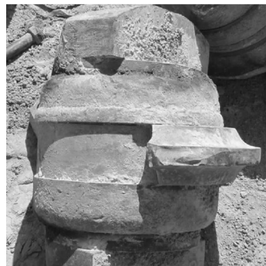
(c) 刀圈断裂
