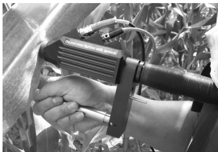
Fig. 1 Spectral measurement on leaf with the plant probe
