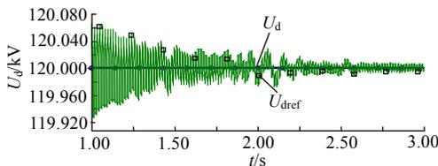
(b) DC voltage results with optimized parameters
