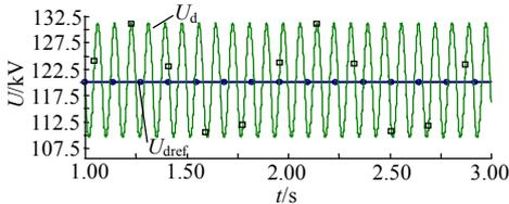
(a) DC voltage results with initial parameters
