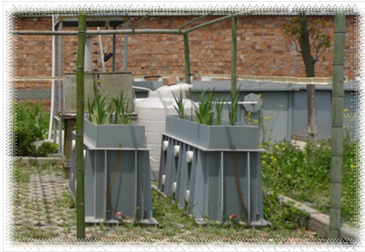
Fig. 1 Subsurface-flow constructed wetland systems and sampling spots location (① indicates sampling location)
